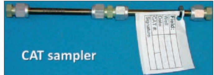
Fig. 3. Picture of a CAT sampler. The length of the sampler is around 20 cm and it weighs below 100 gram.
