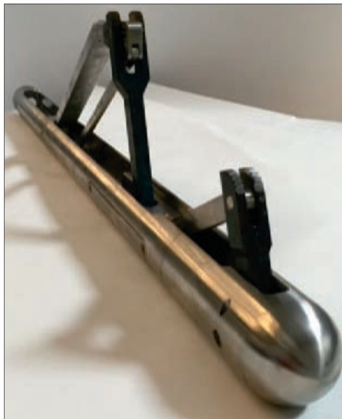
Fig. 5. A 2½" hydraulically powered CT tractor — the eccentric link gripper (ELG) section.
