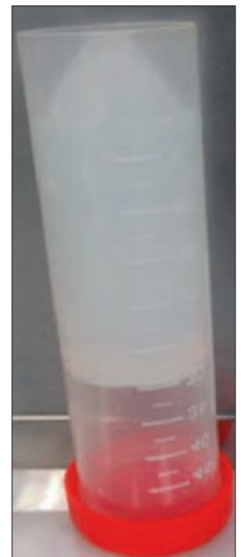
Fig. 5. Representation of the inverted sealed tube test demonstrating gelation under static conditions.
