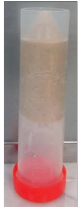
Fig. 7. A representative sand pack consolidated by the cationic nanoparticle treatment fluid.
