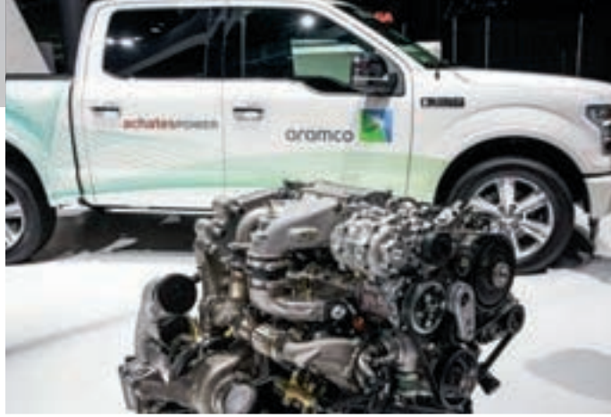
On display at the North American International Auto Show in Detroit is the opposed-piston gasoline compression ignition engine — Saudi Aramco's flagship technology focus.
